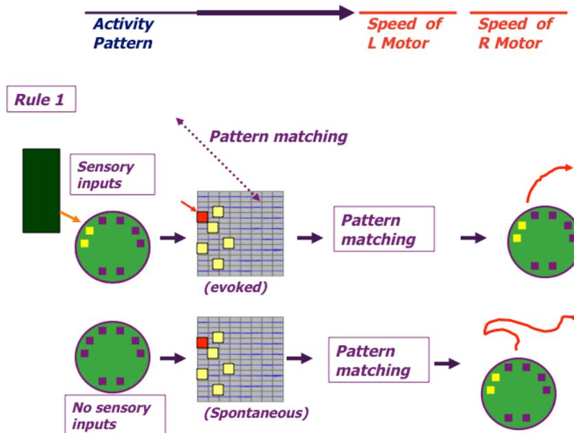
First, the particular patterns of the sensor values of the robot are translated in a stimulation pattern. This stimulation evokes a particular pattern in the LNN, according to that sensor's inputs. The system then recognises this pattern and controls the speed of the actuators to generate the appropriate behaviour by the robot body. For the example in Figure 7, IR sensors detect an obstacle at the left side, so the robot should increase the
