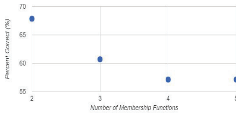
Fig. 3. Number of membership functions per input x parameter. The threshold was 0.1. The tuning variable K_w was 0.1, and both K_a and K_b were 0.01.
