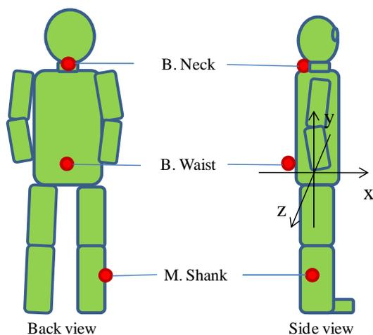
**Fig. 2** Attachment of accelerometers on the body.
