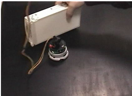
Fig. 5: Collision Avoidance of Robot with Living Neuronal Network
