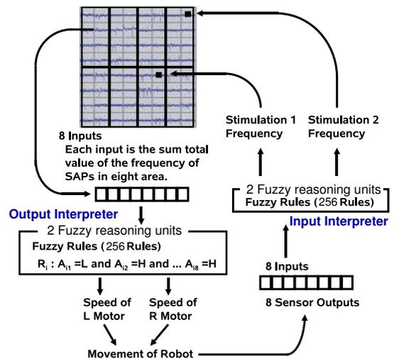
Fig. 2. A direct coupling type of closed-loop interaction.
