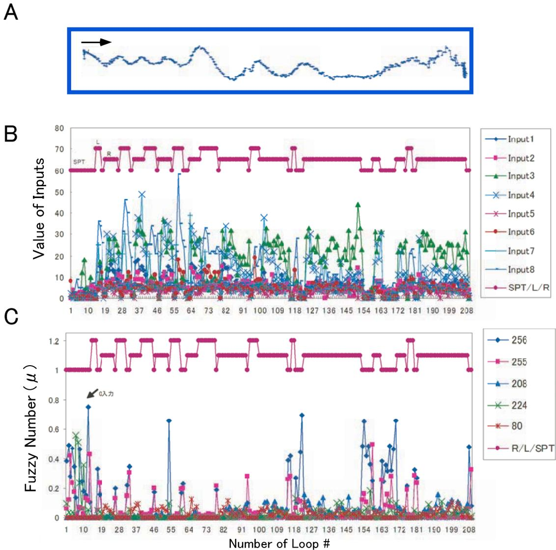
Fig. 6. A. An example of trajectory of Vitoroid robot body. B. Label of classified inputs (L,R,SPT) and number of inputs, corresponding activities in 8 ch electrodes. C. Compatibility degrees of top 5 rules during an experiments. The experiment is same as one indicated in B.
