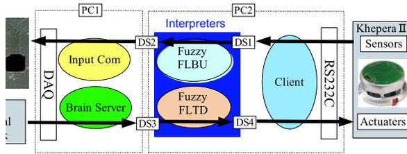
Fig. 3. Schematic diagram of Neuro-Robotic hybrid system. The system consists of 5 independent programs and recording system for multiple-site extracellular potentials, two computers and robot body.
