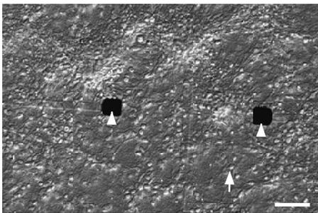
Fig. 1. Example of cultured living neuronal network (E17D10). The white bar indicates 50  $\mu$  m. White arrowheads indicate planar microelectrodes, arranged in an 8 x 8 grid on the culture dish. Example of neuron is indicated (white arrow)
