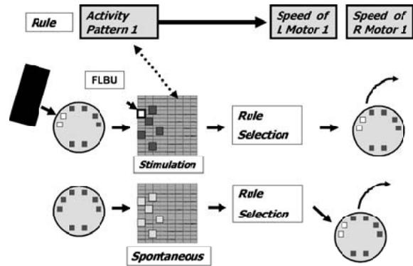
Fig. 4. Spatiotemporal pattern of evoked and spontaneous activity of neuron linked to speed of actuators on a robot body.
